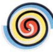
**All Stages Working Together.** During operation, all six gas passages are in various stages of compression at all times, resulting in nearly continuous suction and discharge.
